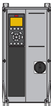
A4 IP55 with mains disconnect
